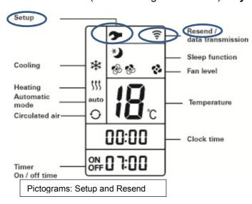
If the Setup pictogram does not flash, a reset must be performed. Slide the bottom cover open and press the Reset button with a pointed object until all the pictograms appear on the display, then release the Reset button.
